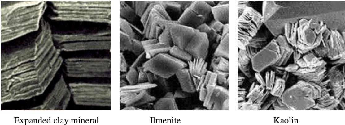
**Fig. 6** Micrographs of different clay minerals.
